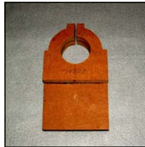
Parts B/D glue together and slot cut into tab located on the top. This slot allows the 3/16 carriage bolt to be tightened and clamps the router onto the unit.
