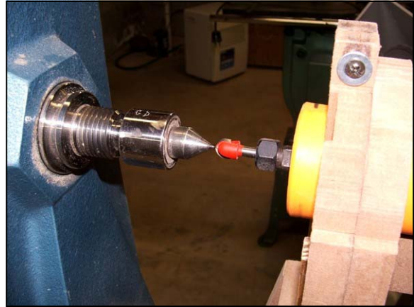
The router bit is centered on the spindle of the head-
