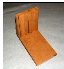
Part C, shows slots dado-ed in the back surface, and slot cut for the adjusting bolt and wing nut. This is glue to Part A. Note: vertical supports. Part A has a scalloped edge on the front. this not critical, space the bumps equal distance apart. The depth of the cut for the bumps is 3/4". These bumps ride along the template that is affixed to the work surface and makes working the router along a curve much easier.
