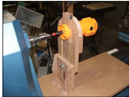
Assembled router jig showing distance from the spindle center to work surface.
